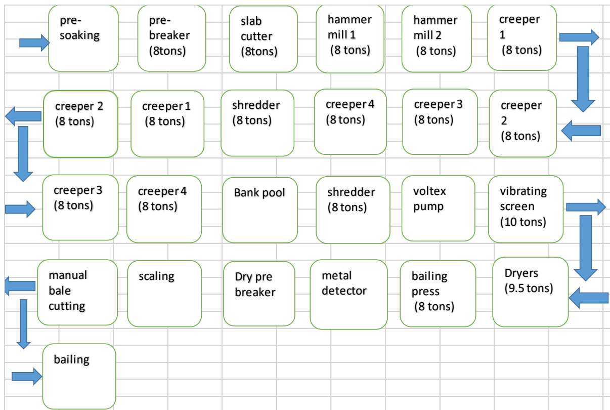
Figure 1: Flow chat for a rubber processing line.
